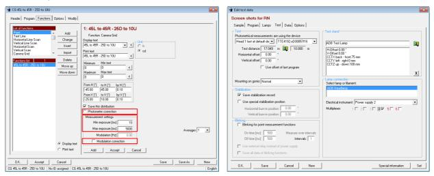
If a *CameraGrid* measurement is part of the program flow, the camera can be chosen in the tab *Test* (right picture above). In addition, a photometer choice is available to define the photometer head to be used for stabilisation, for automatic gradient determination and of course to correct the recorded *CameraGrid* with a photometer measurement.
