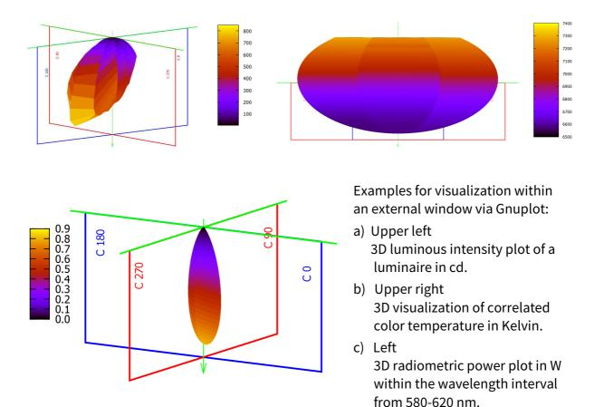
A standard view is implemented by LMT, but customization of visualization parameters via Gnuplot is possible. However, this is left to the individual user. The pictures above illustrate a few examples as outlined in the figure caption.
