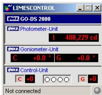
Main window example for general lighting with Goniophotometer GO-DS 2000
